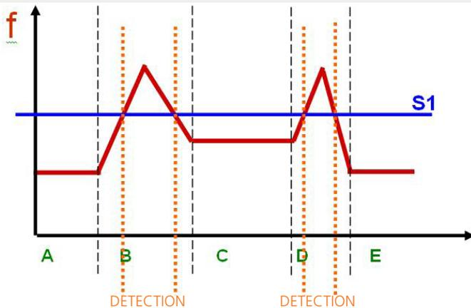
In this application, the sensitivity is adjusted via the potentiometer to the value  $S1$ . This means that every frequency superior to this limit creates detection and therefore relay activation.
