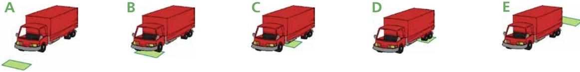
The graphic on the right shows the frequency and induction variations measured by an induction loop detector when a truck passes over a loop. The variation is bigger at cab and axle level (positions B and D), and smaller at trailer level (position C). This observation can be explained by the fact that the trailer is generally higher than the cab (with regard to the ground) and consequently influences the loop induction less.
